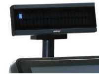
PD-2501 11 mm 2 x 20 VFD display, 5X7 dot matrix, RS232 interface
