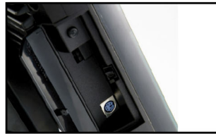
Push-open cover to protect power switch from accidental shutdown of the system, providing extra security to the operation
